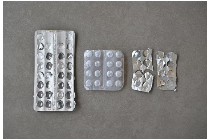
It is difficult to separate the materials in this multi-layer packaging so the strips are usually discarded as general waste. ST PHOTO: LIM YAOHUI
